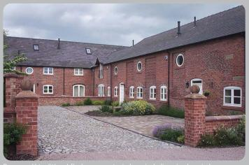
Dempsey V traditional flush casement windows including circular windows with openers - factory finished in microporous white paint.
