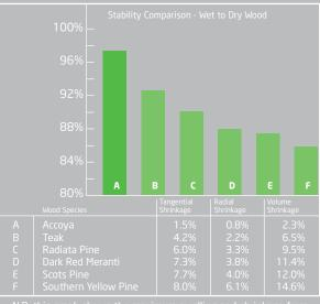
N.B. this graph shows the maximum swelling and shrinkage from fully soaked to oven dry (the most extreme laboratory test). The main data table shows instability in more normal weather conditions (with simulated humidity varying between 60 and 90 percent).
