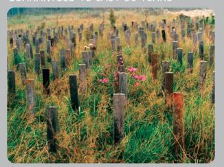
The picture above shows extensive "graveyard" field trials over a 10 year period which demonstrates Accoya™ Class 1 durability rating which exceeds some of the worlds most durable timber species, including Teak.
